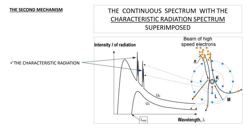
In the produced spectrum of x-rays very sharp spikes appear above the smooth background. These spikes are called *characteristic lines* and the x-radiation is termed *characteristic radiation*.
