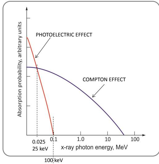
The amount of x-rays absorbed or scattered depends upon how many <u>electrons</u> are encountered along xray's path.
