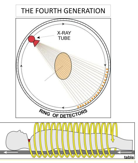
With spiral CT, the patient table advances at a constant rate through the gantry while the X-ray tube rotates continuously around the patient.
