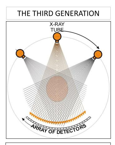
In the "third generation" CT scanner, the rigidly coupled source-detector unit is rotated around the scanned body and yield projection data for different angular positions.
