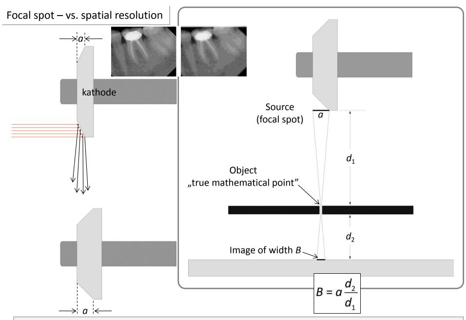
Both, the geometry  $(d_1, d_2)$  and the dimension (a) of the focal spot determine spatial resolution. Under optimal conditions in radiography the spatial resolution reaches 0.1 mm.
