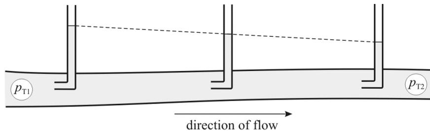
Fig. 4. The flow of real fluid is accompanied by unavoidable drop in the total pressure  $\Delta p_T = p_{T1} - p_{T2}$  along the direction of flow. Thus, to maintain the constant rate of flow a difference in pressures between tube ends is necessary.
