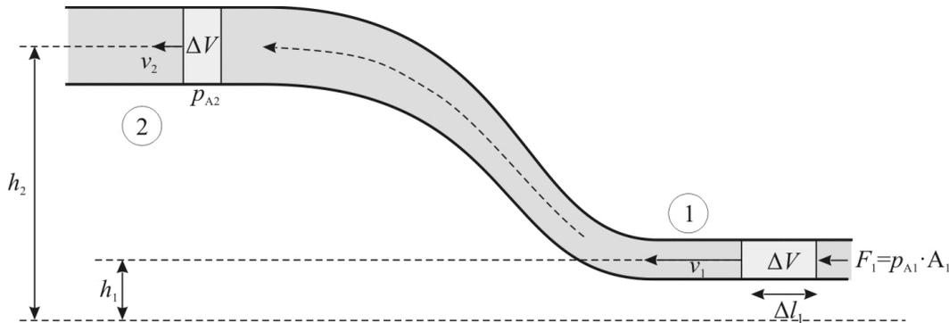
Fig. 2. To increase the mechanical energy of the fluid (the kinetic and potential energy) a force  $F_1$  in section 1 (on the vessel's right side) has to be applied along the distance  $\Delta l_1$ . The amount of work  $W$  done by force  $F_1$  equals:  $W = F_1 \cdot \Delta l_1 = p_{A1} \cdot A_1 \Delta l_1$ , where  $p_{A1}$  is the pressure in section 1 of the vessel of a cross-section area  $A_1$ .
